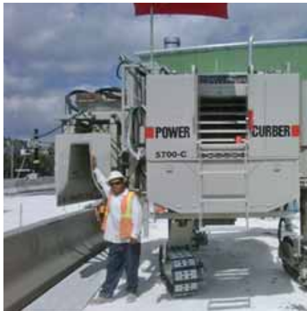
5700-C equipped with Barrier Mold Lift, All Crawler Steering, and Polyurethane track pads.
