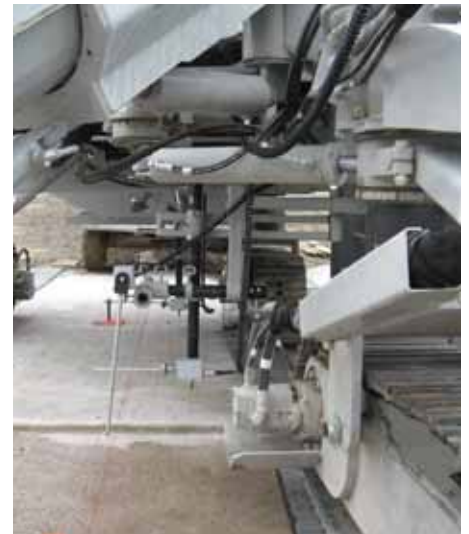
Parapet sensor mounting.
