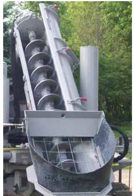
Auger Conveyor; lid opens for cleaning.
