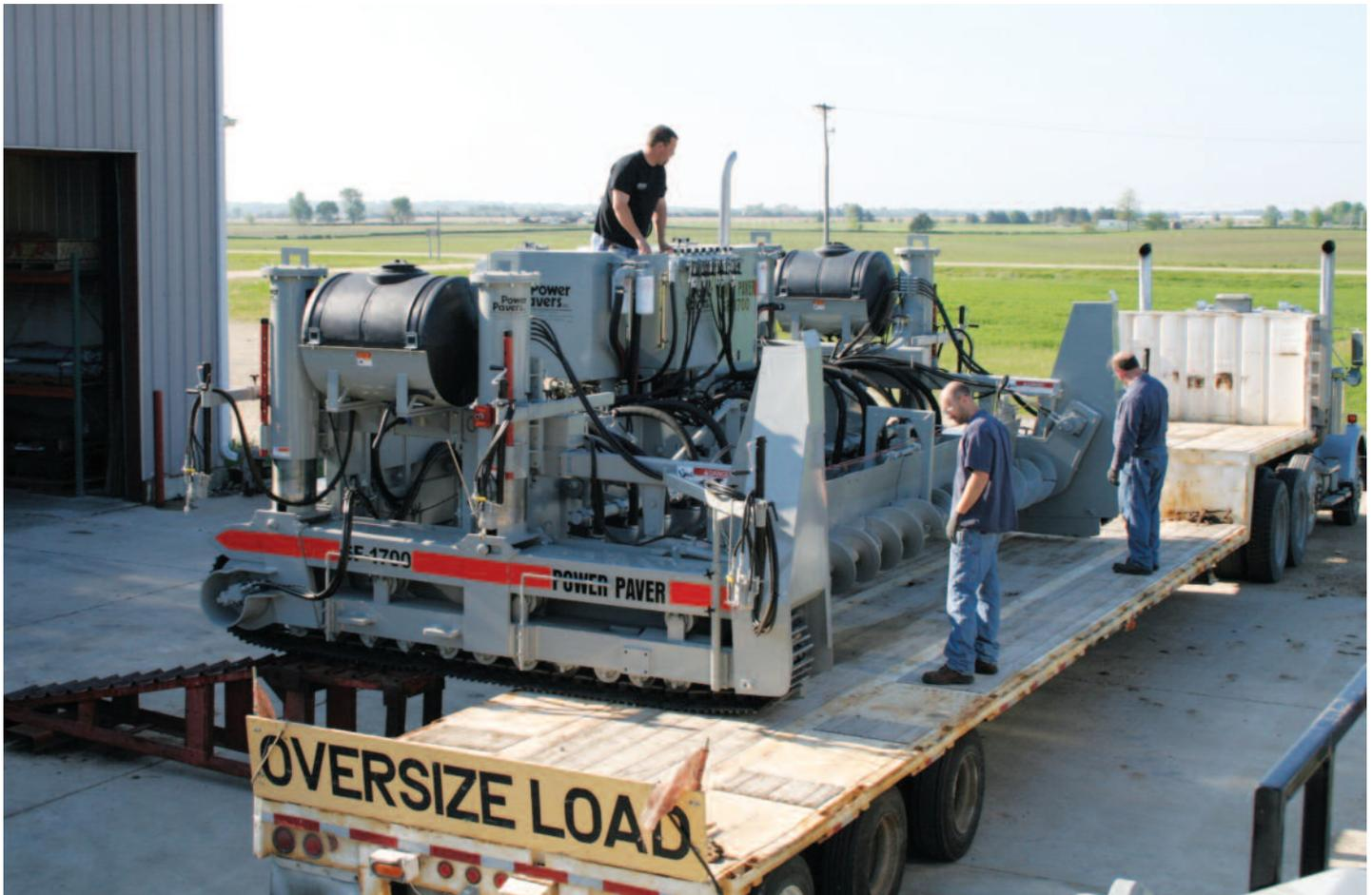
Loading and unloading the SF-1700 and SF-2700 pavers is quick and easy with side ramps.
