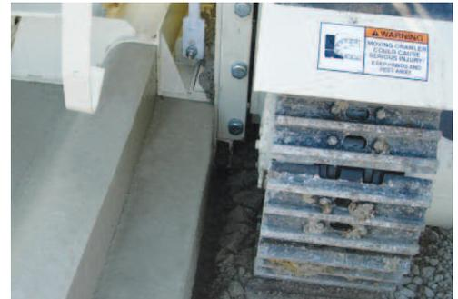
An optional curb mold, even for specialized profiles, can add integral curb to one or both sides of the pavement.
