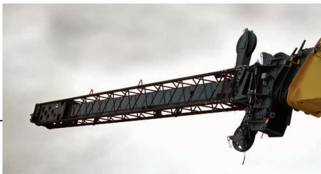
• **Tip Height** – The RT540E offers a 7,9 m - 13,7 m (26 ft - 45 ft) offsettable telescopic swingaway providing a maximum tip height of 47 m (154 ft) with 13,7 m (45 ft).
