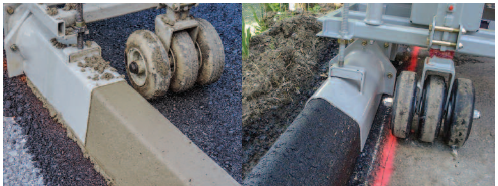
The 150 can be used to pour either concrete or asphalt curb. The pneumatic tires (left) are standard. The hard rubber wheels (right) are an option.
