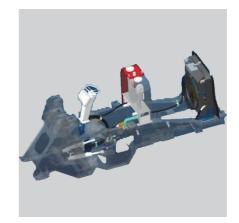
Load sensing steering maximizes machine performance by directing power through the steering system only when needed.
