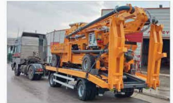
The frame of the FT 208 Trailer can be folded down while being shipped. For overseas shipments, the Scorpion Pump and its carrier trailer can be shipped with the same 40' HC container.
